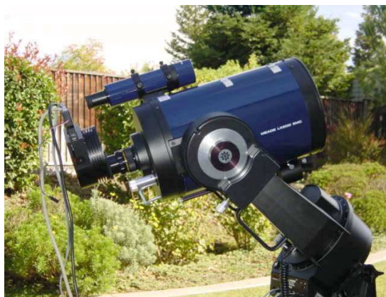
Figure 1. Our prototype Santa Barbara Instruments Group (SBIG) ST-7E CCD and Meade LX-200 8 inch aperture telescope system
